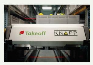
Systems developed by Takeoff Technologies use small shuttles such as the one pictured to move frequently purchased goods through Micro Fulfillment Centers, thereby making it more convenient and cost effective for grocers to engage in e-commerce. *Courtesy Takeoff Technologies*.
