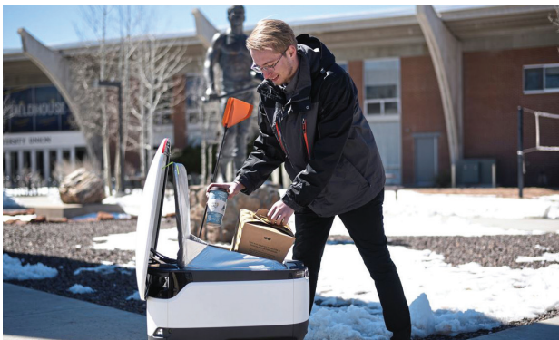
Starship Technologies’ automated package handling and delivery robots are dropped off near customer locations by Robovan delivery vans for autonomous “last block” deliveries. ■
